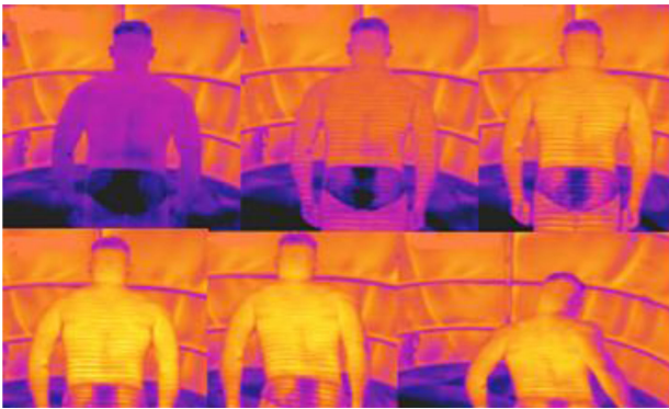
FIGURE 50. Millimeter wave radiation is absorbed by the human skin (0.4-mm thickness) resulting in instant heating as shown in the IR pictures when the back of a target person is radiated (max. effect bottom right). It is uncomfortable but safe and completely reversible in its effects.
